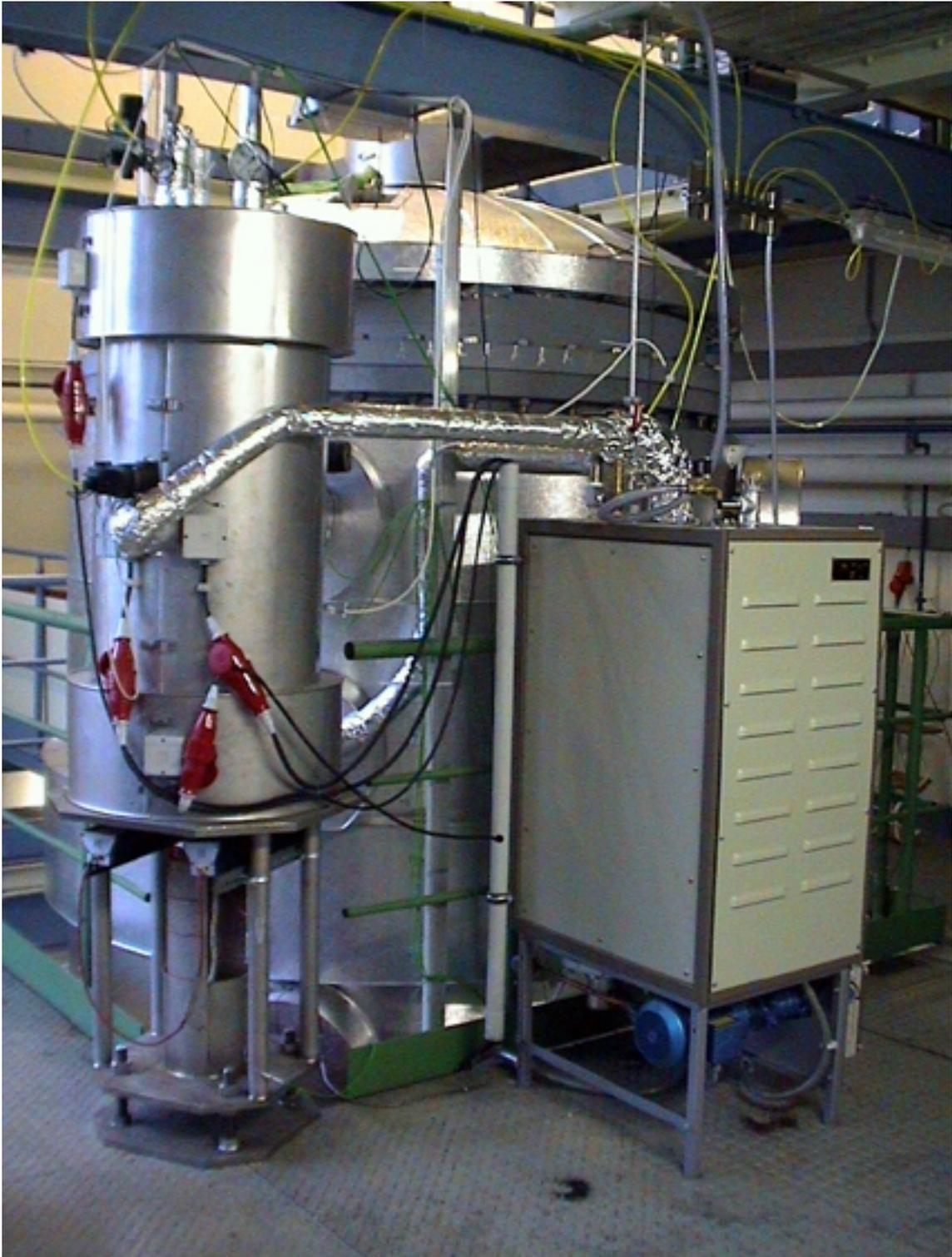
**Fig. 10. The steam accumulator (left) and the steam generator (right)**
