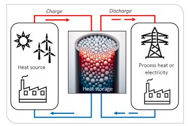
Use of a high-temperature heat storage system to supply process heat or electric power. (Graphics: KIT/KALLA)
