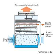
surface and thus extracts heat from the medium in the coil (primary circuit). With this arrangement, temperatures below the ambient air temperature can be achieved up to close to the wet bulb temperature. Dry operation (without secondary circuit) is also possible in cold weather. Finally, the process can be reversed and the device can be used (especially) in winter as an evaporator or heat source for a heat pump.
